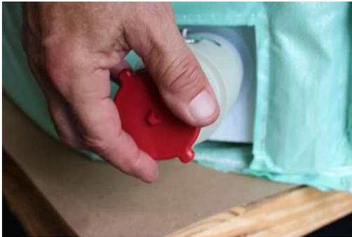
Take the valve and screw it into the discharge gland until the valve is touching the discharge gland. No threads on the valve should be visible. It is helpful to start screwing the valve counter clockwise until the threads align and then turn the valve clockwise until it is touching the discharge gland. You are now ready to discharge the contents.
