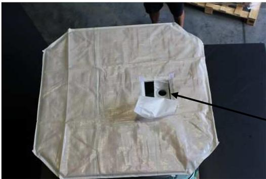
Place the lid partially on top of the IBC leaving room for you to reach under the lid to grab the 2" filling gland on the liner and then pulling through the large square opening in the lid.
