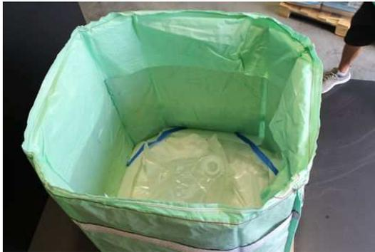
Lower the cassetted liner into the IBC and make sure to align the discharge gland with the opening in the corner of the IBC. Pull the 2" fill gland up towards the top of the IBC.
