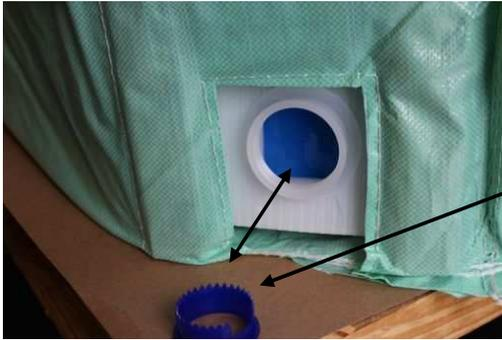
Inside the cap is a blue colored cutting ring. The ring has teeth on one side. Place the ring back into the discharge gland with the teeth facing towards the liner.
