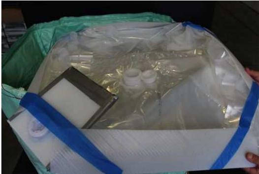
After the bin is set up on the pallet, take the cassetted liner pictured to the right and unscrew the 2" filling cap on the top of the liner.
