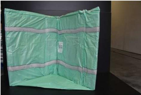
Remove the lid, liner and valve from the top of the collapsed IBC and then stand the IBC upright with the red sewing yarn at the top.
