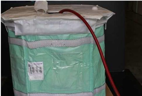
Once the filling gland is secured in the filling bridge in the lid, you are ready to fill your 264 gallon EWS IBC. Using a garden hose, gently lower the garden hose several feet into the liner as pictured to the right. Make sure the portion of your garden hose that will go inside the IBC is clean and sanitized. You will need to lower several feet of hose into the liner to make sure the hose does not come out during the filling process.
