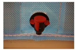
To discharge the water from the EWS bin, you first must rip off the tamper evident tab on the discharge valve.
